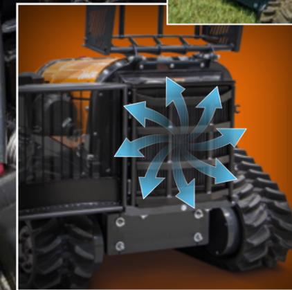
HYDRAULISCHER FLEXXAIRE -UMKEHRLÜFTER
